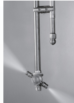
Inside, double nozzle system, orbital and 360°
