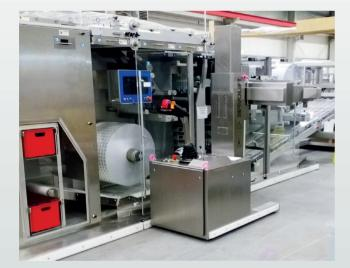
Sideways positioning at the packaging line for exchange of the foil reel
